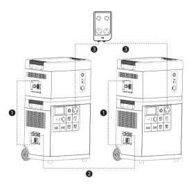
Two MANGO POWER E units can be linked together with an E-Link cable to double the output power and voltage.
